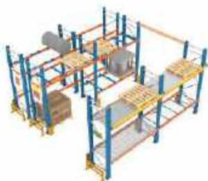
Changing Static pallet racking to Mobile Pallet Racking
